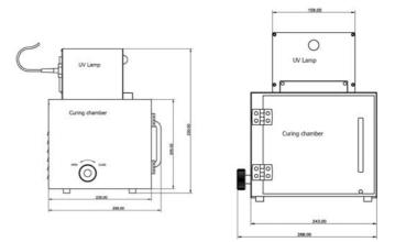
Side view (left) and front view (right) of UVACUBE 100
