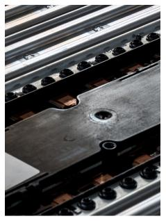
Due to temperature swings, the screws securing the coolant system to the battery pack made noticeable noise during expansion and contraction.
