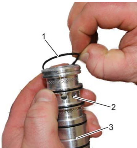
Fig. 44: Detaching the O-rings
