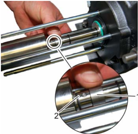
Fig. 83: Securing the dowel pin
