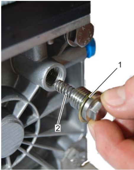
Fig. 54: Fastening the pilot valve
