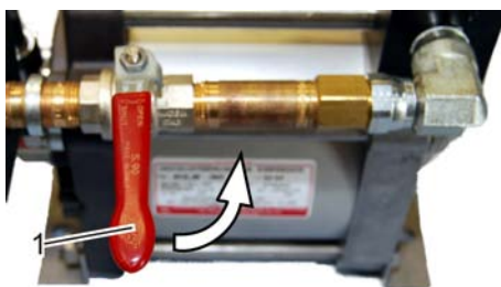
Fig. 27: Opening the ball valve
