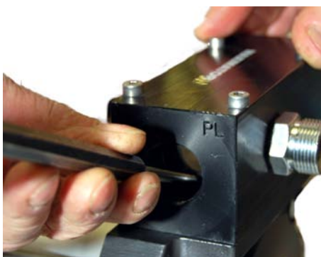
Fig. 42: Punching out the sleeve
