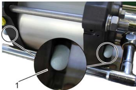
Fig. 15: Removing breather silencer
