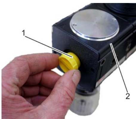
Fig. 12: Unscrewing sealing plug
