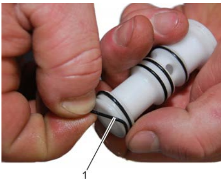
Fig. 35: Sliding on new O-rings
