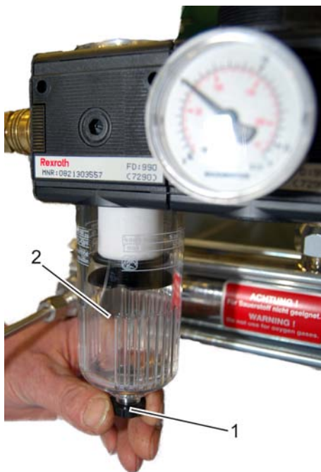
Fig. 28: Checking the water separator
