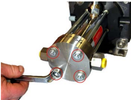
Fig. 57: Undoing the booster head
