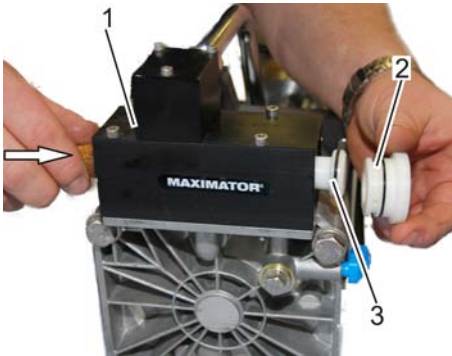
Fig. 33: Removing control valve and cap
