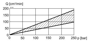
Q = f (I) DNPPM18 Volume flow adjustment characteristics
