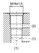
Cavity drawing according to ISO 7789–18–01–0–98
