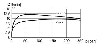
Q = f (I) DOPPM18 Volume flow adjustment characteristics
