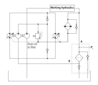
The entire dirt produced in the hydrostatic drive by abrasion is filtered out immediately and is thus not taken in by the pump of the open-loop circuit. This circuit layout is always recommended if the return flow only slightly exceeds the suction flow, i.e. if there is a risk that the 0,5 bar precharging pressure cannot be maintained.
