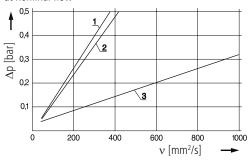
Pressure drop as a function of the **flow volume** at  $v = 35 \text{ mm}^2/\text{s}$  (0 = casing empty)
