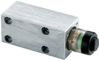
**Function:** When the preset differential pressure is reached, the optical indicator changes from green to red. If the pressure differential returns to a value below the preset limit, the indicator changes back to green, i.e. no manual reset of the indicator is required.
