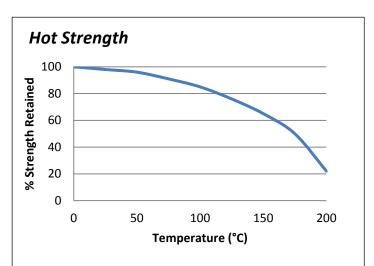
"Hot strength" shear strength tests performed on mild steel. Fully cured then conditioned to pull temperature for 30 minutes before testing. ES5691 can withstand higher temperatures for brief periods (such as for paint baking and wave soldering processes) providing the joint is not unduly stressed. The minimum temperature the cured adhesive can be exposed to is -40°C (-40°F) depending on the materials being bonded.
