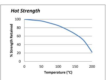
"Hot strength" shear strength tests performed on mild steel. Fully cured then conditioned to pull temperature for 30 minutes before testing. ES568 can withstand higher temperatures for brief periods (such as for paint baking and wave soldering processes) providing the joint is not unduly stressed. The minimum temperature the cured adhesive can be exposed to is -40°C (-40°F) depending on the materials being bonded.
