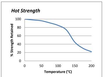
"Hot strength" shear strength tests performed on mild steel. Fully cured then conditioned to pull temperature for 30 minutes before testing. ES561 can withstand higher temperatures for brief periods (such as for paint baking and wave soldering processes) providing the joint is not unduly stressed. The minimum temperature the cured adhesive can be exposed to is -40°C (-40°F) depending on the materials being bonded.
